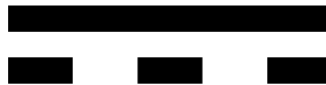
FIGURE 3: THE GRAPHIC ABOVE INDICATES THAT THE CUBE ACTS AS A DIRECT CURRENT SUPPLY
