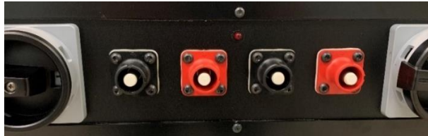
FIGURE 11: FEED FRONT PANEL WITH GROUND FAULT INDICATOR LED
