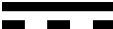
FIGURE 3: THE GRAPHIC ABOVE INDICATES THAT THE CONVERTER ACTS AS A DIRECT CURRENT SUPPLY.
