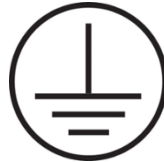
FIGURE 1: THE GRAPHIC ABOVE INDICATES THAT THE FEED IS A GROUNDING CONDUCTOR.
