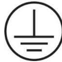
FIGURE 1: THE GRAPHIC ABOVE INDICATES THAT THE BOX IS A GROUNDING CONDUCTOR
