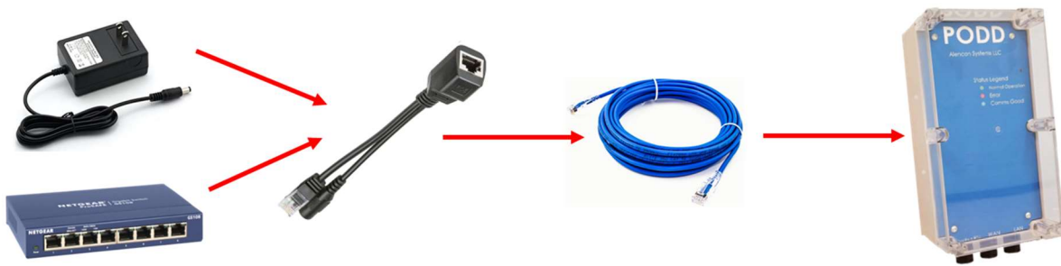
Figure 15: POE Injector with PODD Lab Setup
