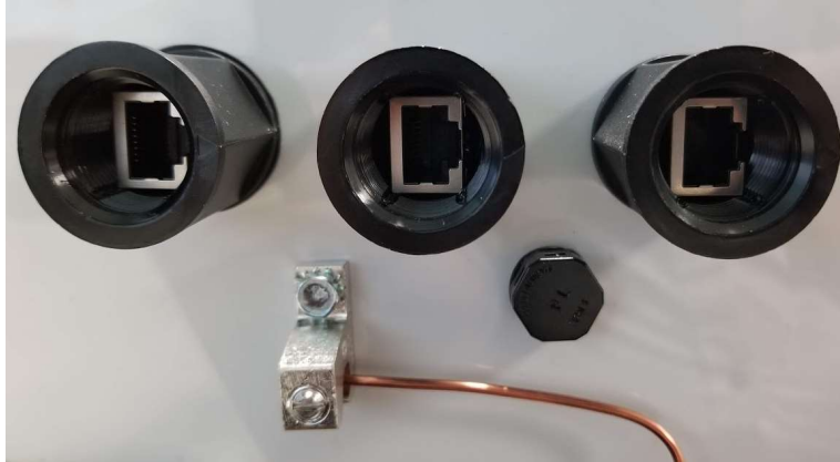
Figure 12: Ground lug placement
