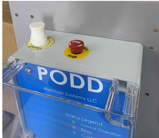
Figure 20: PODD Integrated E-Stop Button
