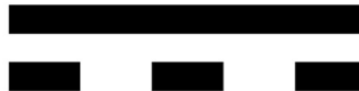
FIGURE 3: THE GRAPHIC ABOVE INDICATES THAT THE BOSS ACTS AS A DIRECT CURRENT SUPPLY
