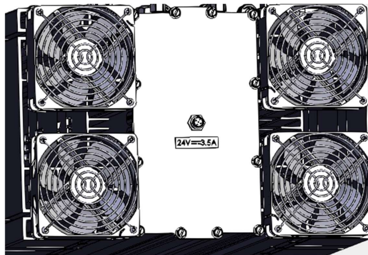
FIGURE 10: BOSS EXTERNAL 24V SUPPLY CONNECTOR (RECEPTACLE SIDE)
