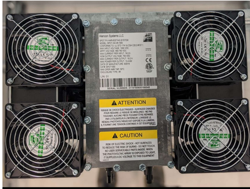
FIGURE 19: SPOT BOTTOM END PLATE WITH COMMENSURATE LABELS
