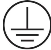
FIGURE 2: THE GRAPHIC ABOVE INDICATES THAT THE SPOT IS A GROUNDING CONDUCTOR.
