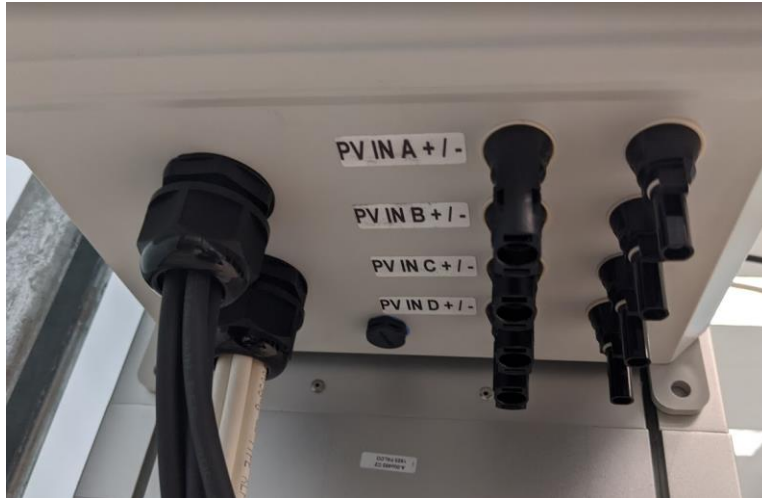
FIGURE 11: BOTTOM VIEW OF AID, INPUT PORTS
