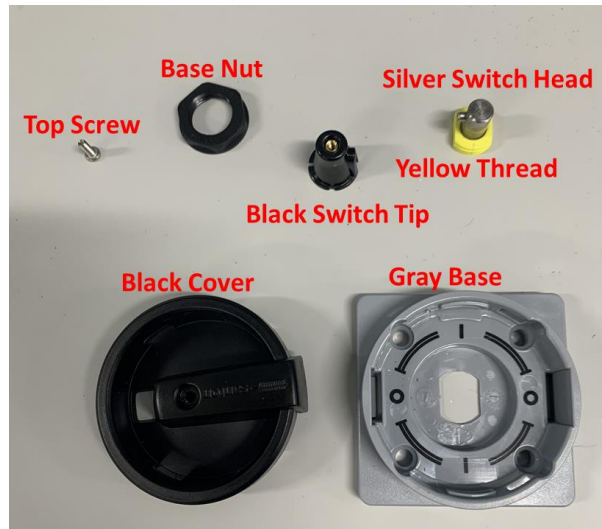
FIGURE 13: DISCONNECT SWITCH COMPONENT PARTS
