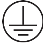
Figure 1: The graphic above indicates that the BOSS or SPOT is a grounding conductor.
