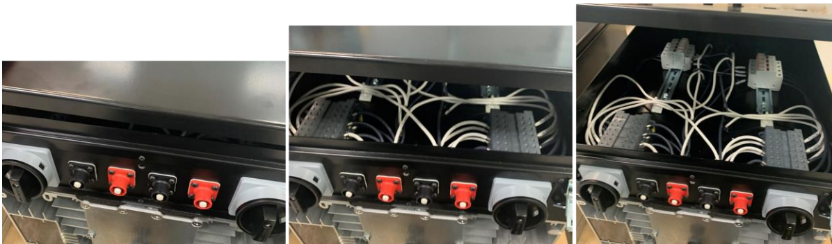
Figure 14: Removing the FEED Cover
