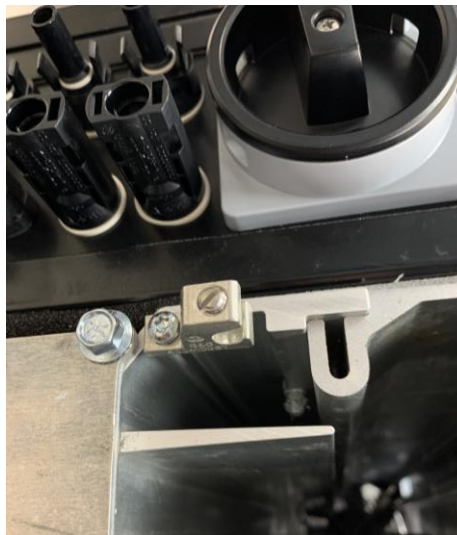
Figure 2: Ground Lug located on the BOSS or SPOT Unit with FEED
