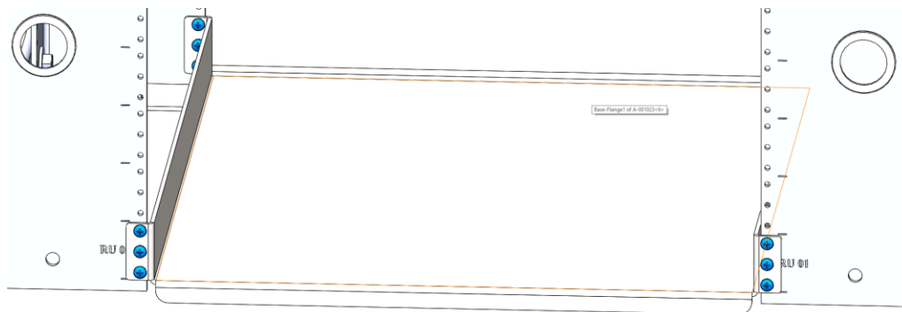
FIGURE 11: TYPICAL SHELF MOUNTING WITH HARDWARE
