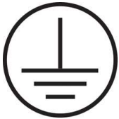
Figure 2: The graphic above indicates that the GARD is a grounding conductor.
