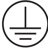
Figure 2: The graphic above indicates that the BOSS is a grounding conductor.
