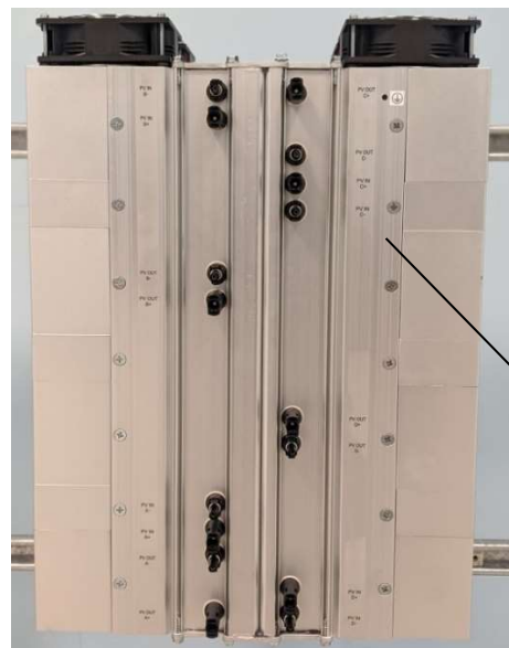
FIGURE 14: SOLAR POWER OPTIMIZER AND TRANSMITTER (SPOT) – VERTICAL MOUNT
