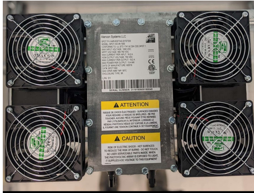
FIGURE 19: SPOT BOTTOM END PLATE WITH COMMENSURATE LABELS
