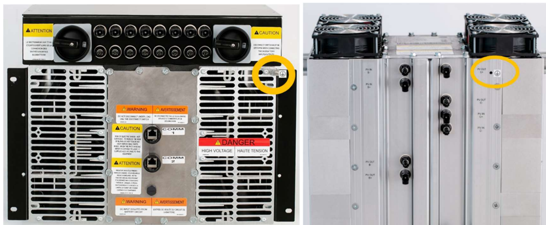
FIGURE 24: SPOT GROUND LUG LOCATION EXAMPLES (IN ORANGE)
