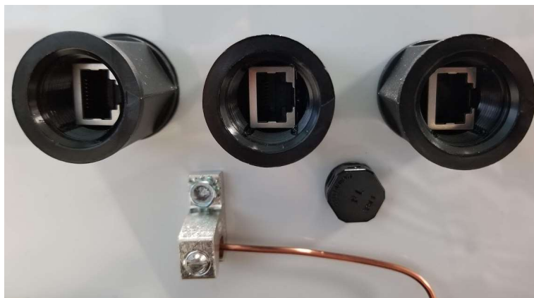
Figure 14: Ground lug placement
