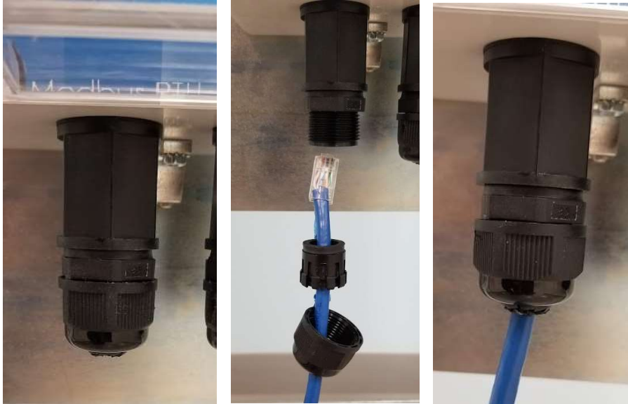
Figure 15: Water-proof wiring on the PODD
